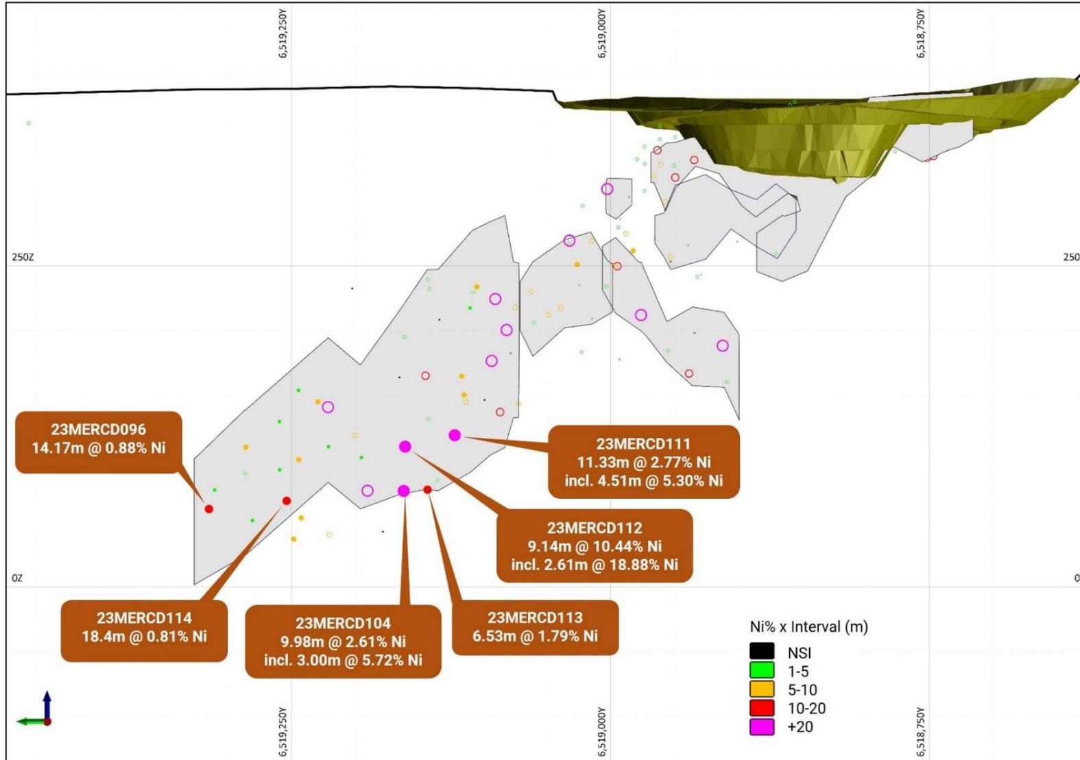
**Figure 6:** 132N Longsection looking East. Existing open pit and 2020 MRE wireframes (grey), nickel % x interval meters solid symbol 2023 drilling, hollow symbol = historic drilling results
