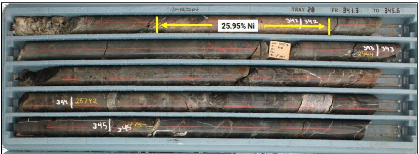
**Figure 3:** 23MERCD104 displaying massive sulphide mineralisation grading at 25.95% Ni
