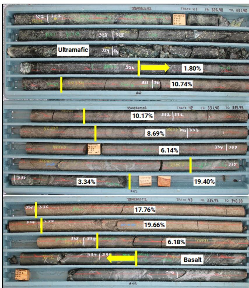
Figure 2: 23MERCD112 displaying individual Ni assay results from disseminated to massive sulphide mineralisation.
